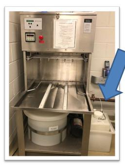
The stand-alone tank is a 5-gallon carboy. To avoid air bubbles in the line the carboy should never be allowed to empty. It is recommended to not allow carboy to go below 2 gallons. The carboy is marked for a visual reminder of when to fill.
