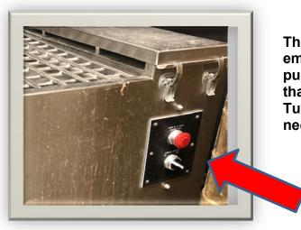
There is an emergency Stop push-button (red) that will stop the Tunnel washer if necessary.
