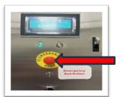
■ In case of emergency Prress the Red Emergency button which is located on the clean and dirty side of the cage wash
