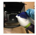
Position the fogger nozzle inside the room to be decontaminated close to the room entry door approximately one foot away from the wall on a level surface.
