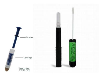
Insert the cartridge into the preprogrammed handheld ATP monitoring device, making sure that the correct collection site/surface is selected as applicable. Once the cartridge is inserted, close the door to initiate reading.
