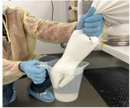
5.If bubbles are present in the jar with Quatricide or soapy water, then the glove is broken. Immediately tie the glove by using vinyl tape.
