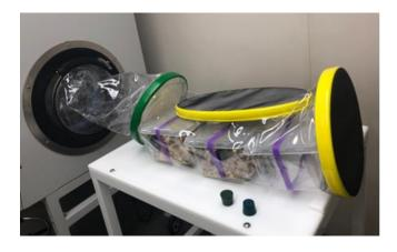
14. The sterile operator will take off the inner port cap inside the BSC.
