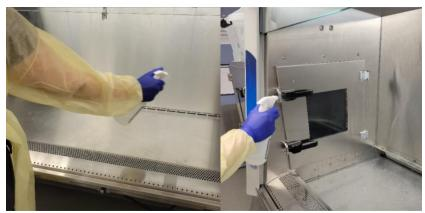
7. Remove the BSC surface panels by pushing down the latch in the hood and lifting the middle surface sheet up toward the back of the hood. Latch the middle sheet up.
