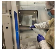
11. Spray the inside of the BSC with sterile cleaning water, saturating the areas that have excess Clidox. Make sure to spray under the grille and any other hard to reach areas. Wipe with paper towels.
