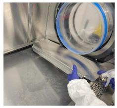
10. Open the internal TC door and spray the inside of the door with sterile cleaning water. Make sure to saturate small areas where Clidox can reside, especially around the gasket. Wipe with paper towels. Close the internal TC door once it is dry.
