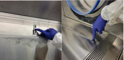
8. Spray the underneath of the middle surface panel with sterile cleaning water and wipe using paper towels.
