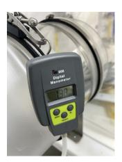
3. The isolator is inflated through the other nipple in the cap using the compressor and the atomizer without Clidox solution until the gloves are completely inverted and are standing out from the isolator horizontally.
