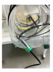
9. Using the atomizer, spray the isolator gloves, inside the inlet and outlet air filter openings, and around the glove rings and the junction of the chamber and port. Hold spray atomizer close to joints to blow sterilant thoroughly into all joints. All surfaces should be saturated.
