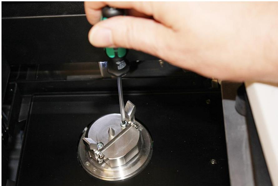
Now you can install sample changer to your scanner. Remove the changer from transportation box. Top lid can be packed separately or just stay on the top of the changer: be careful not to drop it down. Take changer by one hand using handle on the back black part of the changer and by other hand on the slop in the bottom of the column of the changer:
