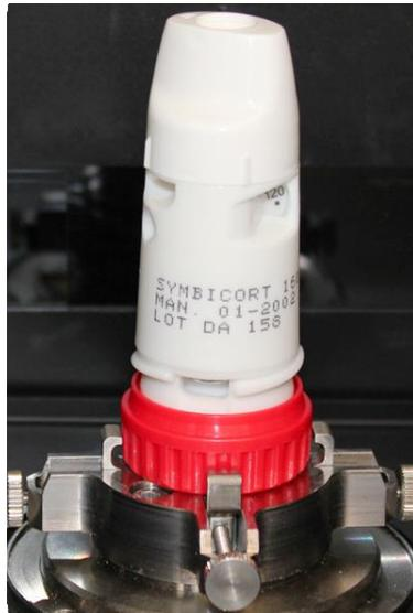
To install steel sample mount use supplied screwdriver. Firstly select angular position of the mount to be sure that connector on the turntable targeted towards milled cavity in the bottom of the mount and afterwards put it coaxial to turntable and secure by two supplied screws:
