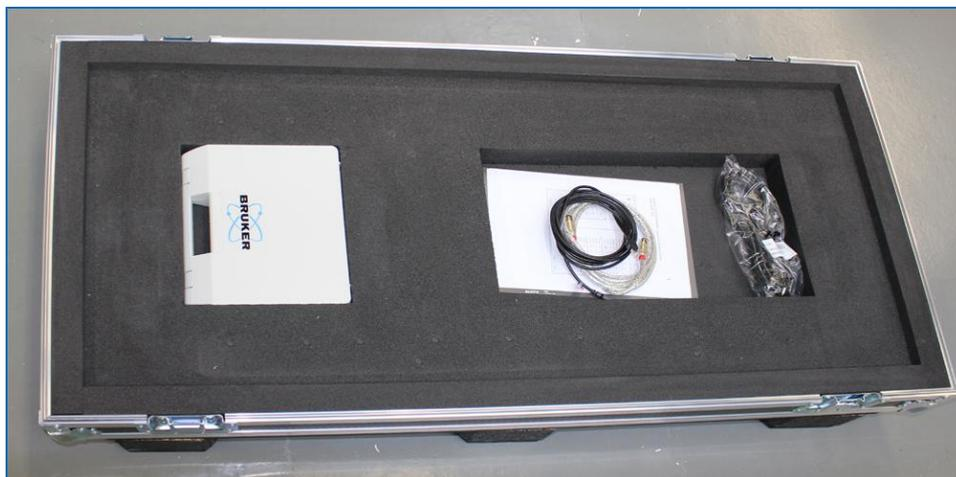
Keep the flightcase for possible moving of the scanner to another location or for sending it back for service or repair.
