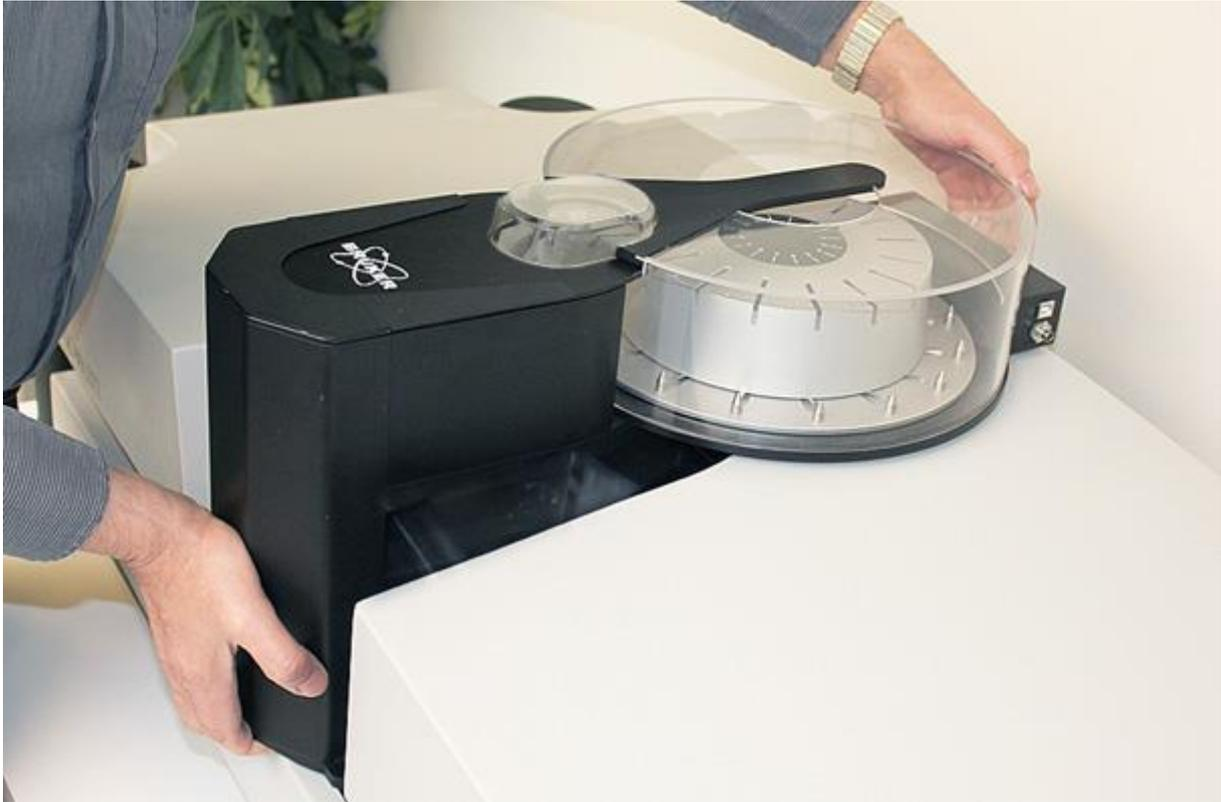
Slide it in parallel to the top surface of the scanner towards the back wall to reach connection of the fork under the changer's carousel with centering pin installed to the scanner. In the proper installation the changer should stay exactly in the middle of the opening of the specimen chamber in parallel to the top surface of the scanner with 2-5mm gap between bottom of the changer carousel and the top surface of the scanner enclosure:
