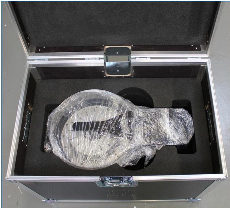
To remove the changer use two round holes in the plastic foam to put your hands under the neck of the changer in the middle of the case. The changer is relatively light and can be handled by one person.
