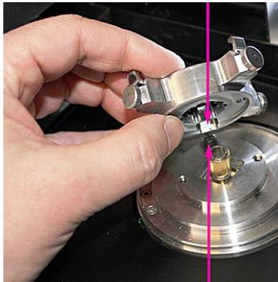
Then attach the holder to the specimen stage and tighten the two screws by supplied screwdriver:
