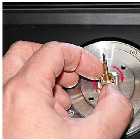
For large objects one can use a supplied steel sample mount. This mount has a chuck with four independently adjusted jaws to hold the objects with complex shape and to adjust their proper centring:
