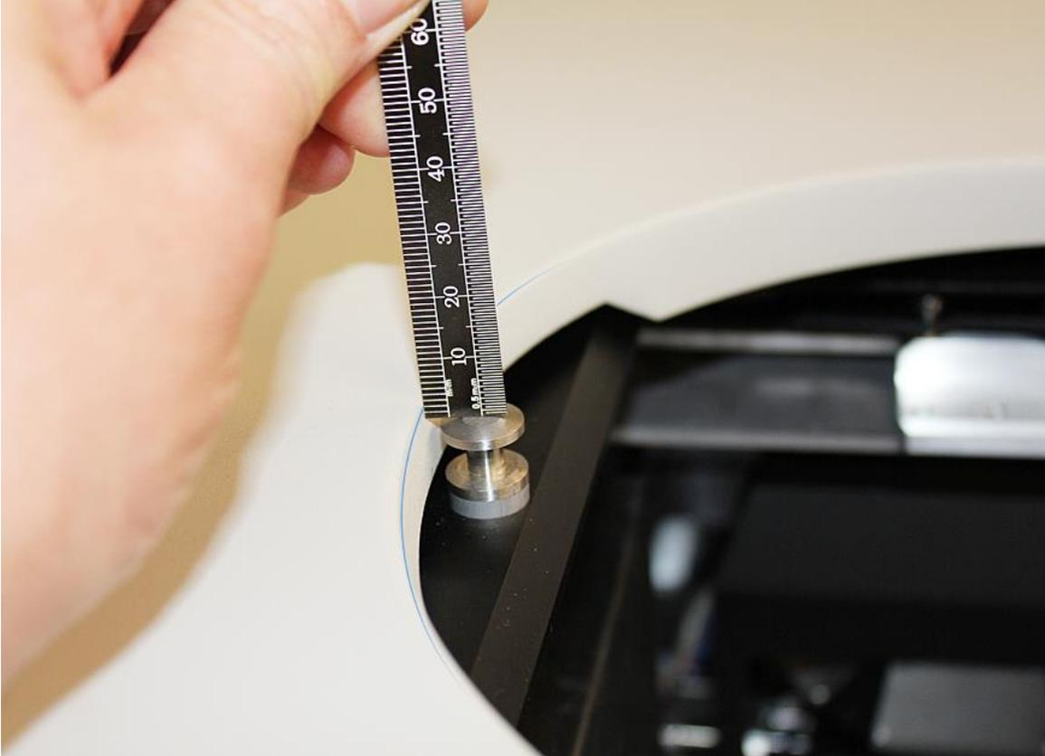
Remove landing pad with two screws from the toolbox and install it to the scanner by following way: firstly adjust angular orientation of landing pad by such way that connector in the object stage inside the scanner will be positioned against milled cavity on the bottom of landing pad:
