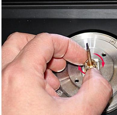
For large and/or asymmetrical samples one can use steel sample holder with 4-jaw chuck. Firstly find such orientation of the holder which will get black connector on the object stage positioned against milled space on the holder:
