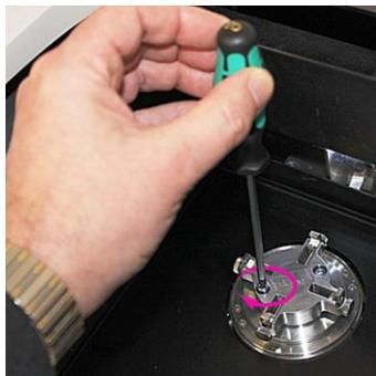
Before closing specimen chamber check that no objects are left on the black plate in the bottom of the chamber. Any object left on this plate will damage your scanner during specimen chamber closing.
