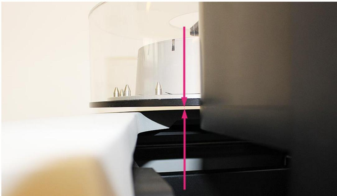
Be sure that two round extensions on the bottom plate of the changer column fit round milled cavities on the front plate of the scanner. Shake a little bit the column of the changer to get both legs properly inserted:
