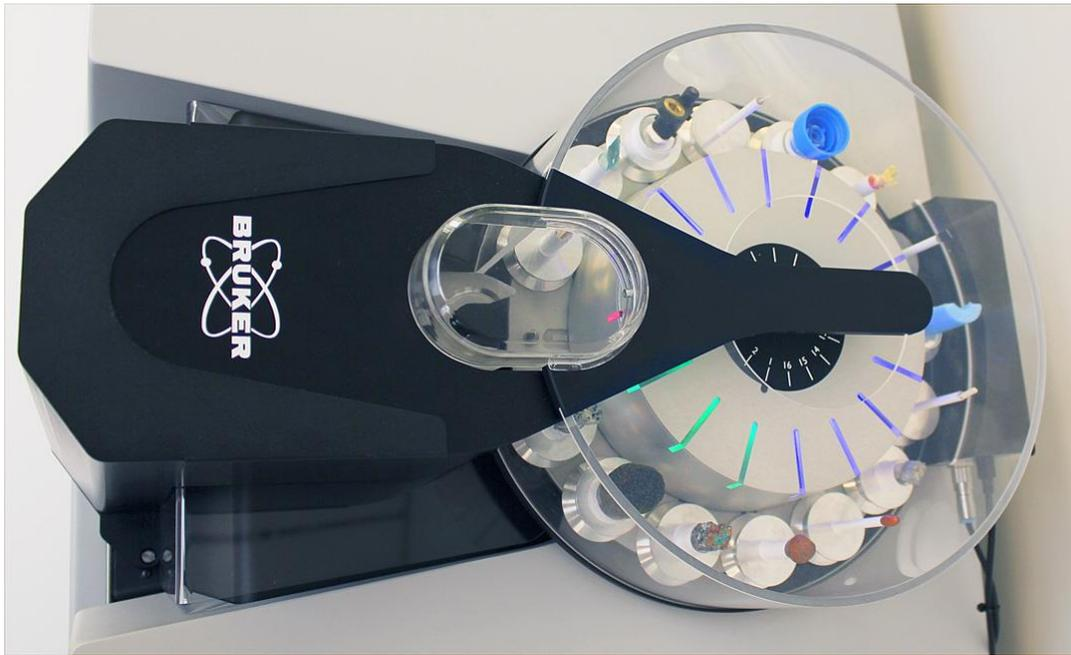
Attention! Never install new sample in the empty position, which is indicated in red because automatic procedure to return sample after scanning to this position will damage the sample changer by collision of the sample mounts.
